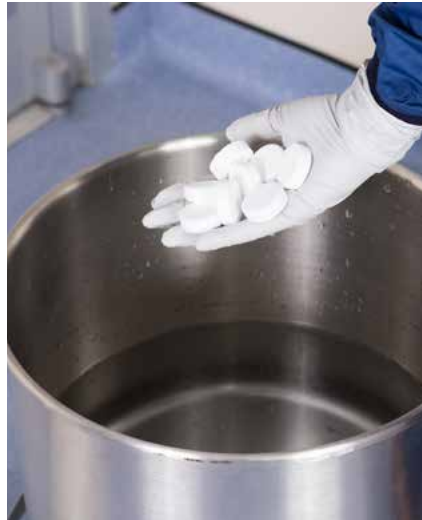
Add 4 tablets per gallon of water to make a sporidical dilution. See the dilution chart on page 16.
